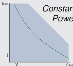
Constant power mode simulates a load whose power consumption is independent of the applied voltage. This is true of many types of equipment that incorporate switchmode regulators.
