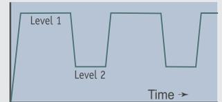
Slew rate control applies to all changes of level including remote control and manual changes between level A and level B.
