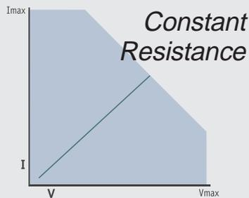
Constant resistance mode simulates a standard resistive load by providing a current drain proportional to voltage. Settings are displayed in Ohms or milli-Ohms.
