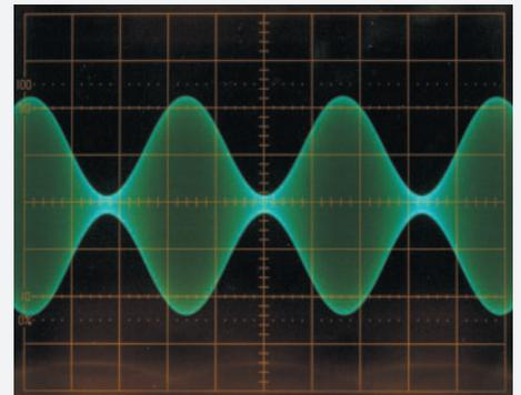
Amplitude modulation using an external sine wave modulation source.
